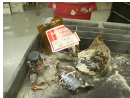
Post explosion of Piranha Solution
