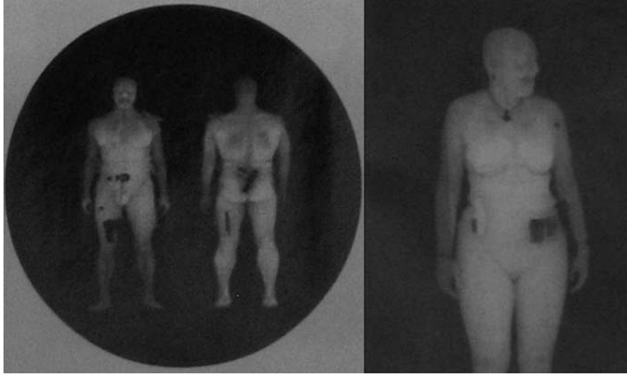
Figure 1 The 3D holographic imaging systems can detect contraband beneath clothing, yet they raise privacy concerns due to the detailed human figure that is revealed.
