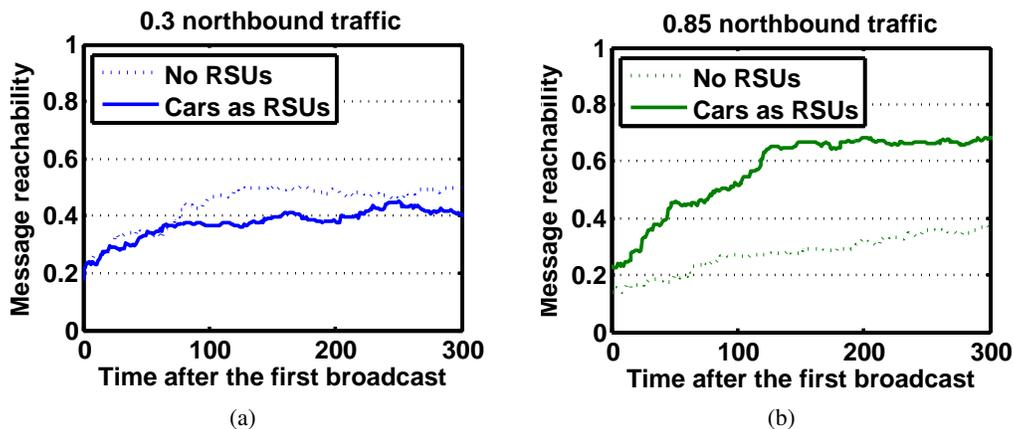
Fig. 5. Impact of the mobility pattern on the message reachability of the network with and without RSU-vehicles. The improvement of RSU-vehicle scheme over the conventional scheme increases with the increase in northbound traffic. The results are based on a 1 km x 1 km Region of Interest network with vehicle density of 100 veh/km<sup>2</sup>, 20% DSRC penetration rate, and 30-second RSU-vehicle stop time.
