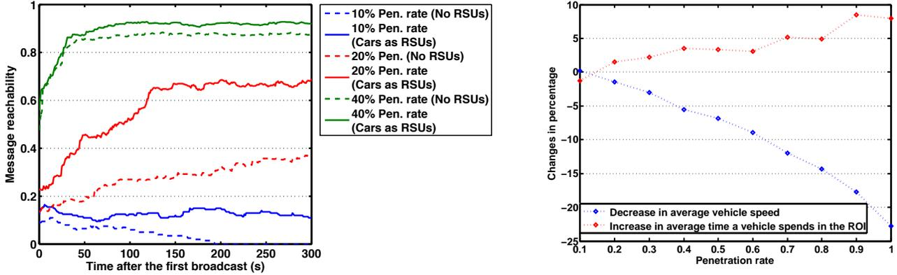
Fig. 3. Impact of vehicle density on the message reachability (left figure) and average vehicle speed and average time a vehicle spends in the ROI (right figure) when the proposed scheme is implemented. Substantial improvement is observed only in sparse and moderately-dense DSRC-equipped network. The results are based on a 1 km x 1 km Region of Interest and 30s of RSU-vehicle stop time.
