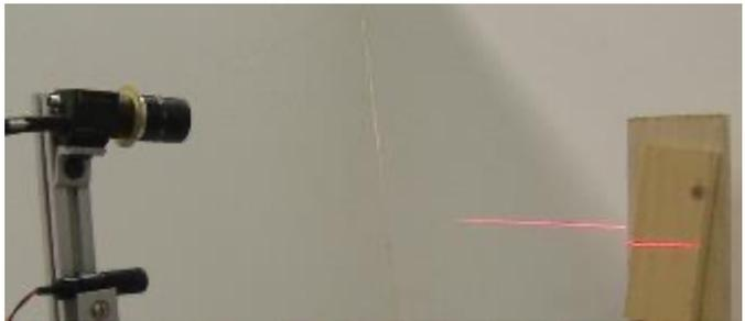
Mount a structure light sensor (cost ~\$1k, resolution ~1mm) on vehicles that regularly traverse the road network .
