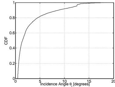
Figure 5: CDF of incidence angle  $\theta_i$  for Porto Open Space dataset. Effective antenna heights of transmitter and receiver: 1.55 m and 1.57 m, respectively.
