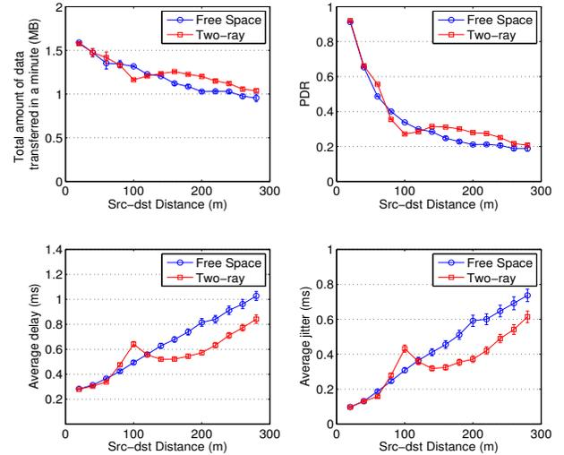
Figure 10: Application performances in terms of throughput, packet delivery rate, latency, and jitter when different LOS channels are used. The standard deviation of fading: 5.3 dB.
