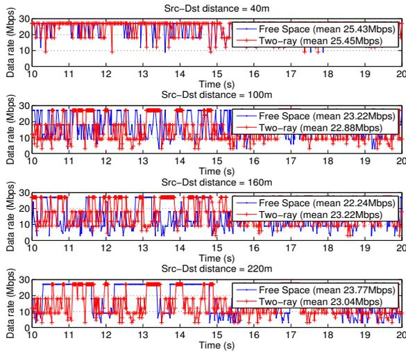
Figure 9: Instantaneous data rate used to transmit a packet for a given distance when the standard deviation of fading is 5.3 dB.
