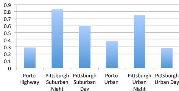
Figure 1: Measured proportion of LOS links in different environments.
