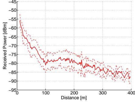
**Figure 3: Received power in the Porto Open Space dataset. Measurement data is placed in two meter distance bins. Only bins with more than 40 data points are included. Dashed red lines represent one standard deviation around the mean received power for each bin.**
