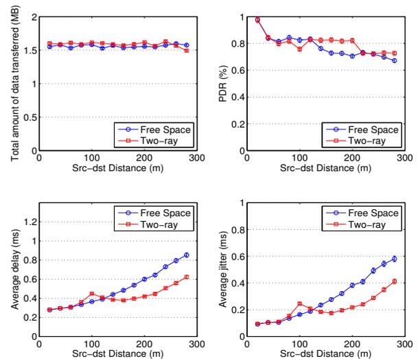
**Figure 8: Application performances in terms of throughput, packet delivery rate, latency, and jitter when different LOS channels are used. The standard deviation of fading: 3.3 dB.**
