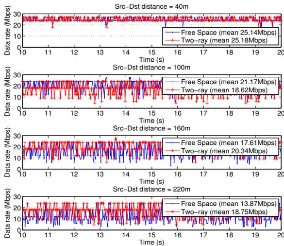
**Figure 7: Instantaneous data rate used to transmit a packet for a given distance when the standard deviation of fading is 3.3 dB.**
