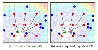
Fig. 2: Trajectories for the integrator model of §III with our controller and different choices for f. We also superimpose the level sets and gradient field of the cost  $\varphi$ .
