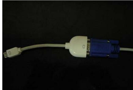
**Illustration 10:** *Plug the video cord into the bigger end of the connector*
