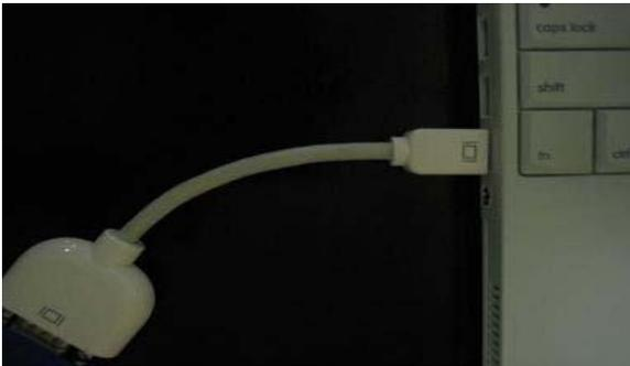
**Illustration 11:** *Plug the smaller end of the connector into the video output slot on your laptop*
