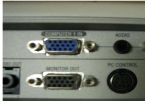
**Illustration 6:** Plug the video cord into Computer 1 slot on the projector
