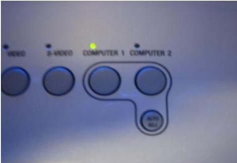
**Illustration 7:** After pushing the “Computer 1” button, the light above it should turn green
