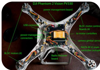
Simpler and cheap components in drone
