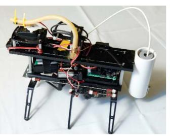
This Trinity Fire Fighting Home Robot Contest entry is a clever design that mounts a gas jet extinguisher on a hexapod platform.
