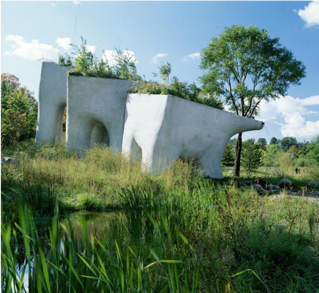
Unique aesthetic markers: Elevated Wetlands, by artist Noel Harding, is a functional ecological art installation along the Don River in Toronto. Water polluted from urban runoff is pumped through the large sculptures using solar energy and cleansed naturally by bacteria in a mini-wetland environment before being returned back to the Don River. Photo courtesy of City of Toronto Archives.
