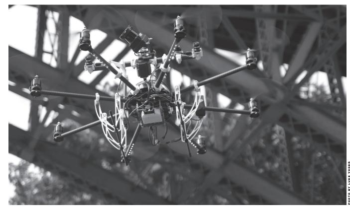
Among the new projects is an autonomous, low-flying robot with 3D imaging that will provide safe, efficient and high-precision assessment of critical infrastructure.
