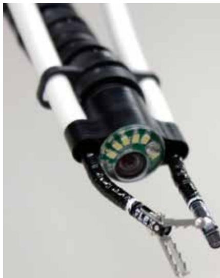
PROFESSOR HOWIE CHOSET'S WORK LED TO THE DEVELOPMENT OF THE FLEX ROBOTIC SYSTEM, WHICH ENABLES SURGEONS TO ACCESS AND VISUALIZE HARD-TO-REACH LOCATIONS THROUGH THE MOUTH.
