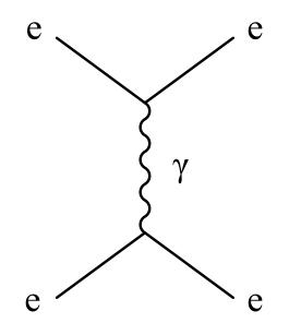
Electromagnetic force between two electrons result exchange of a photon Exchange as local interactions two  $e-\gamma$  interactions
