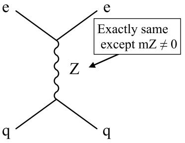
Electron high probability to emit Z when:  $E \times r < h/c$  (consistent with  $\Delta E \Delta t > h$ ) r < h/Ec  $r < h/\sqrt{(pc + mzc^2)c}$ when  $p \rightarrow 0$  then  $r \rightarrow \sim 1/mZ$   $F (= -\Delta p)$  on q cannot extend to  $r = \infty$ Mass of Z makes weak force short ranged.
