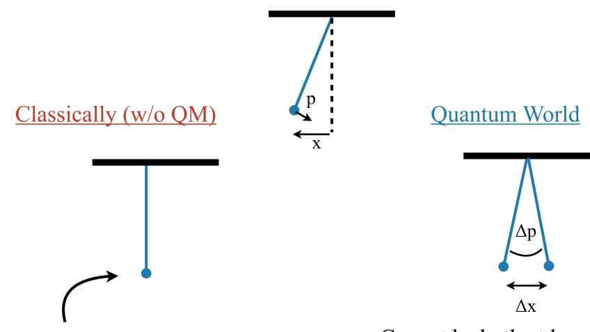
Lowest possible energy is 0. Not moving and at lowest point. Cannot be both at lowest point and not moving.Minimum non-zero energy: E~hω
