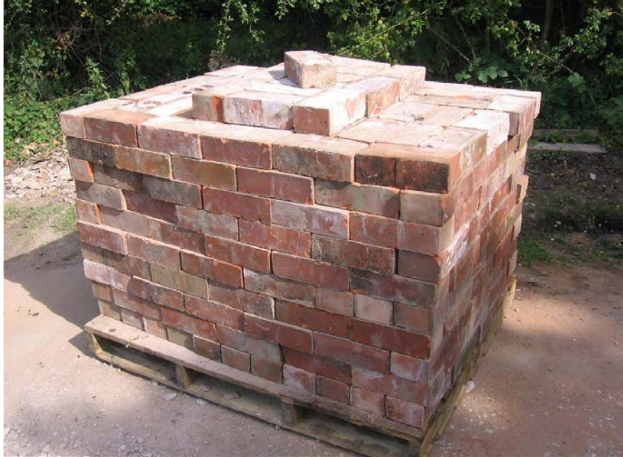
Image 6: A brick pallet, shown above, requires 4 x 4 feet, and it can cost less than $300 to clean and assemble historic bricks for storage
