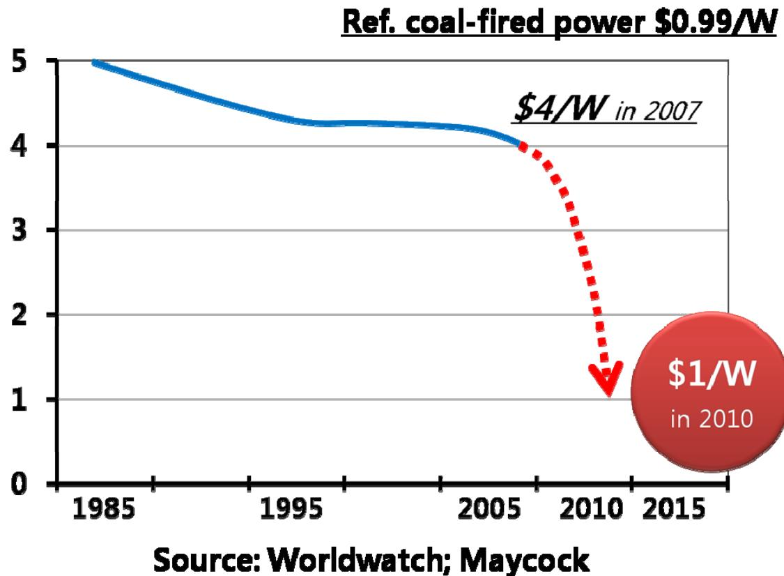
**Figure** Average cost per watt of PV module 1975-2006.
