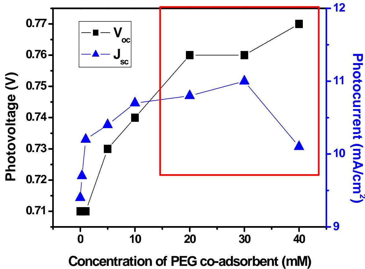
J-V Data of DSSCs as a Function of Concentration of PEG-Based Co-Adsorbent
