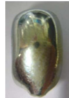
PbTe with  $\text{Bi}_2\text{Te}_3$  ingot
