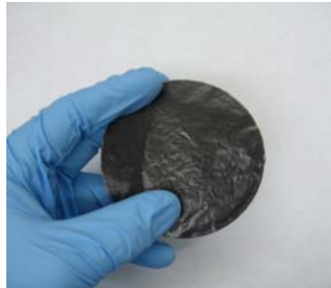
SWCNT paper that is used to make an anode
