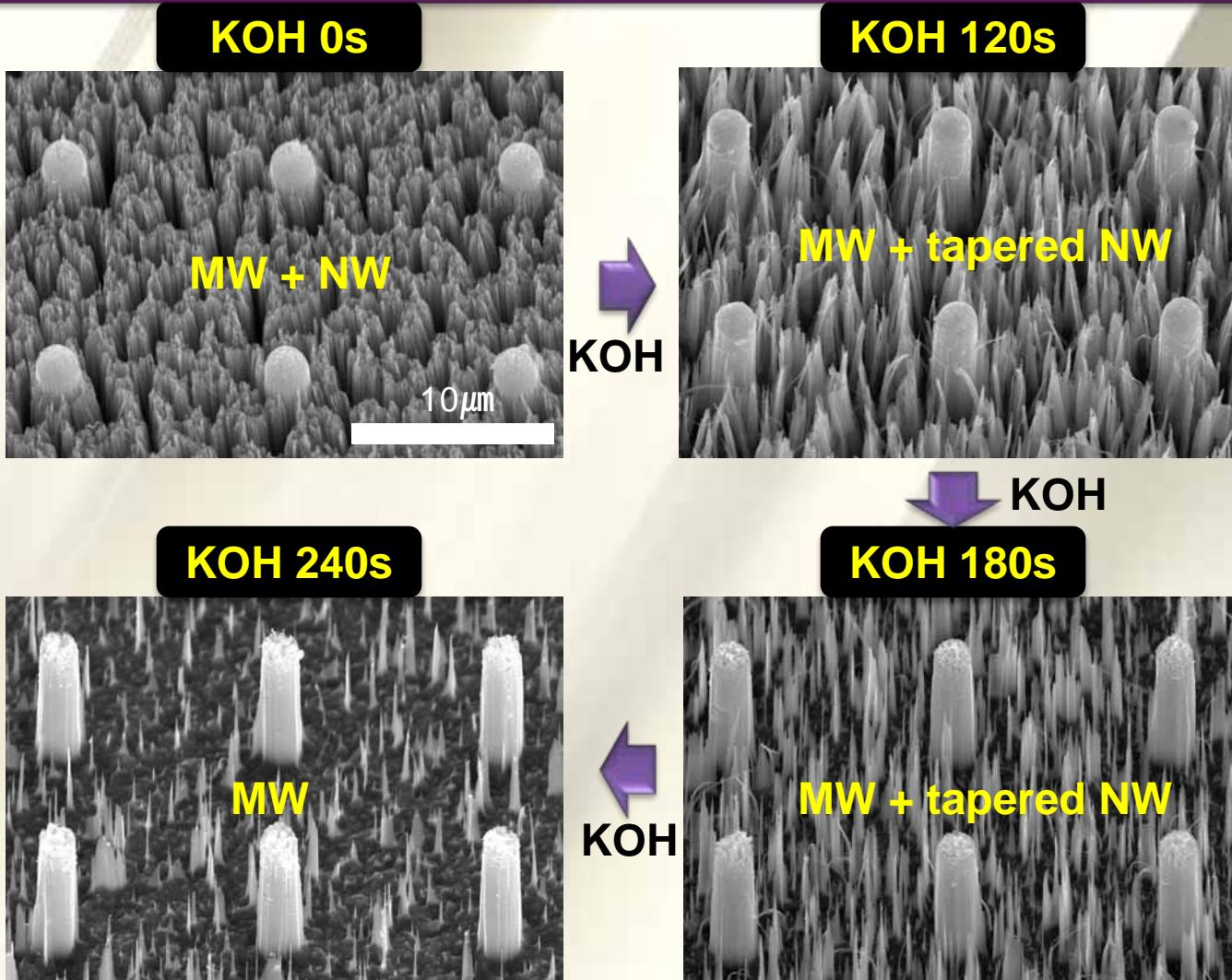
KOH etching could reduce the areal density of NWs while improving the surface roughness of NW.
