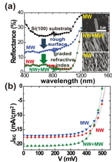
Fig. 8 (a) Optical reflectance data of a polished Si(100) substrate, a sole array of MWs, a sole array of tapered NWs, and a co-integrated structure of MWs and tapered NWs. (b) Their I-V characteristics.
