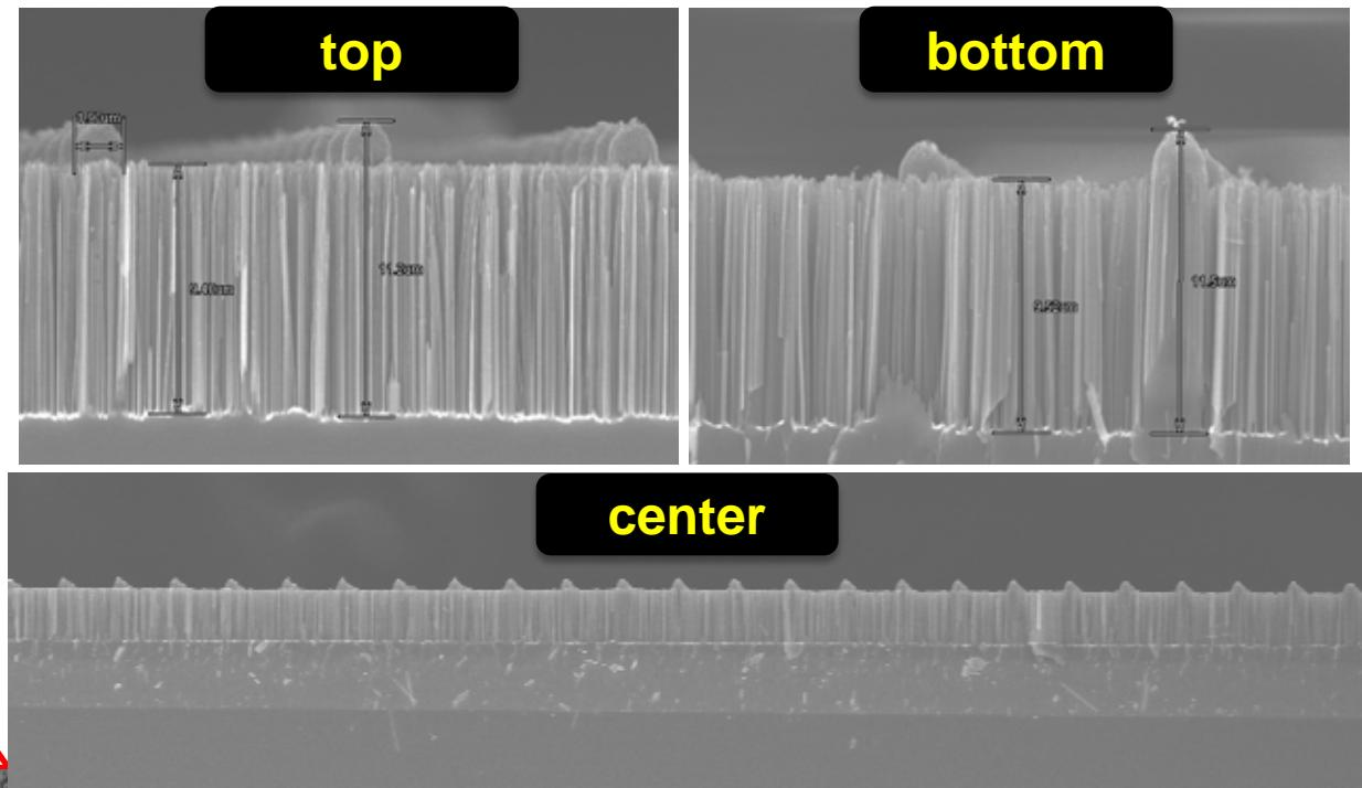
Waferscale co-integrated SiNW+MW arrays show the black color due to excellent absorption.
