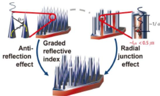
Fig. 1 Conceptual schematic of a novel PV nanodevice based on the co-integration of tapered Si NWs and MWs.
