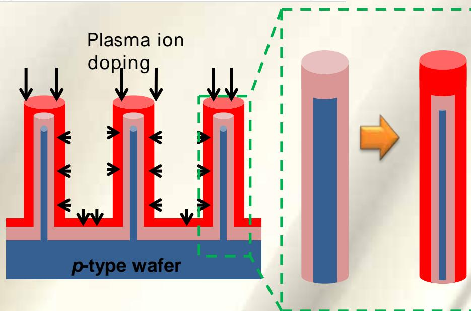
•Intensifying the N+-level of the MW shells while enabling **shallow, conformal doping**
