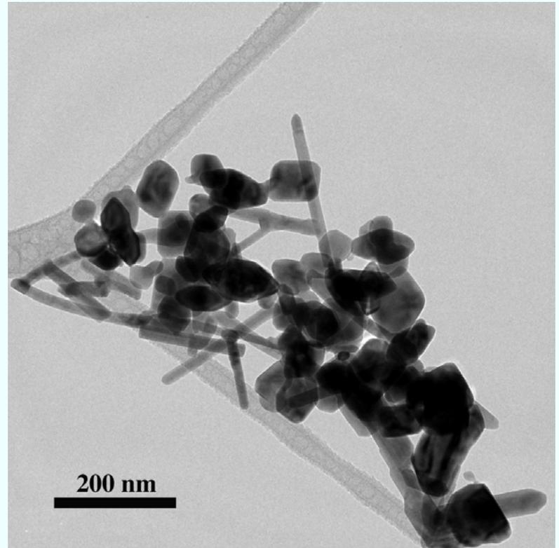
**Synthesis at 150 torr 4% O<sub>2</sub> in Ar, filament temperature ~ 2000 °C. Nanoparticles are observed at high density with the furnace at either 300 or 600 °C. Slightly larger particles observed at higher temperature.**
