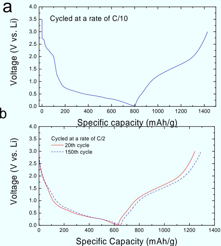
A negative electrode fabricated with MoO<sub>3</sub> crystalline nanoparticles showed a reversible capacity of approximately 630 mAh/g.
