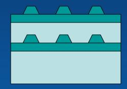
• 3D island formation is driven by a reduction in strain energy that outweighs the increase in surface energy that occurs
