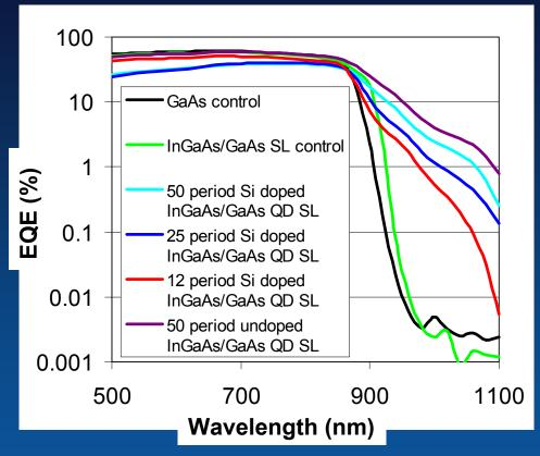
Current generated by absorption of sub-bandgap photons associated with VB-to-IB transition in QDs
