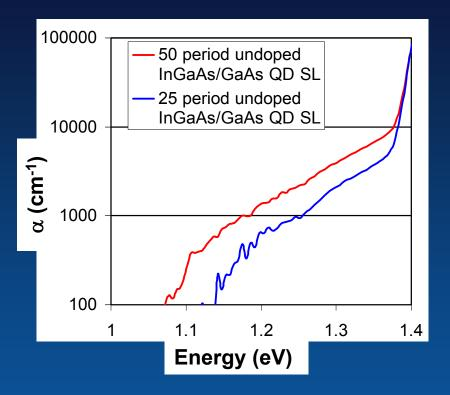
Absorption of subbandgap photons associated with VB-to-IB transition in QDs
