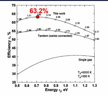
FIG. 2. Efficiency limit for a solar cell with an intermediate band and for a two-terminal ideal tandem cell, in both cases vs the lowest band gap  $\epsilon_I$ , and for a cell with a single band gap. The corresponding values of the highest band gap in cells with intermediate band  $(E_G)$  and in tandem cells  $(E_C)$ , for maximum efficiency, are also presented.
