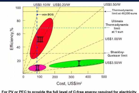
For PV or PEC to provide the full level of C-free energy required for electricity and fuel—solar power cost needs to be ~2 cents/kWh (\$0.40/W<sub>p</sub>).
