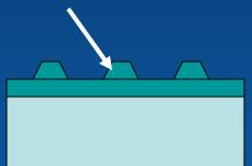
If barrier layers are thin, strain coupling results in vertical stacking of subsequent QD layers
