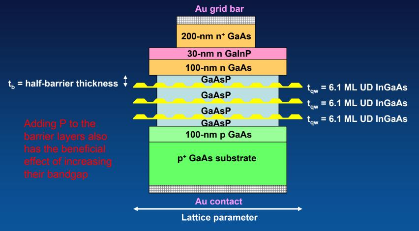
Compressive strain of InGaAs QD layers is compensated by tensile GaAsP layers such that average lattice parameter of QD SL is equal to GaAs substrate
