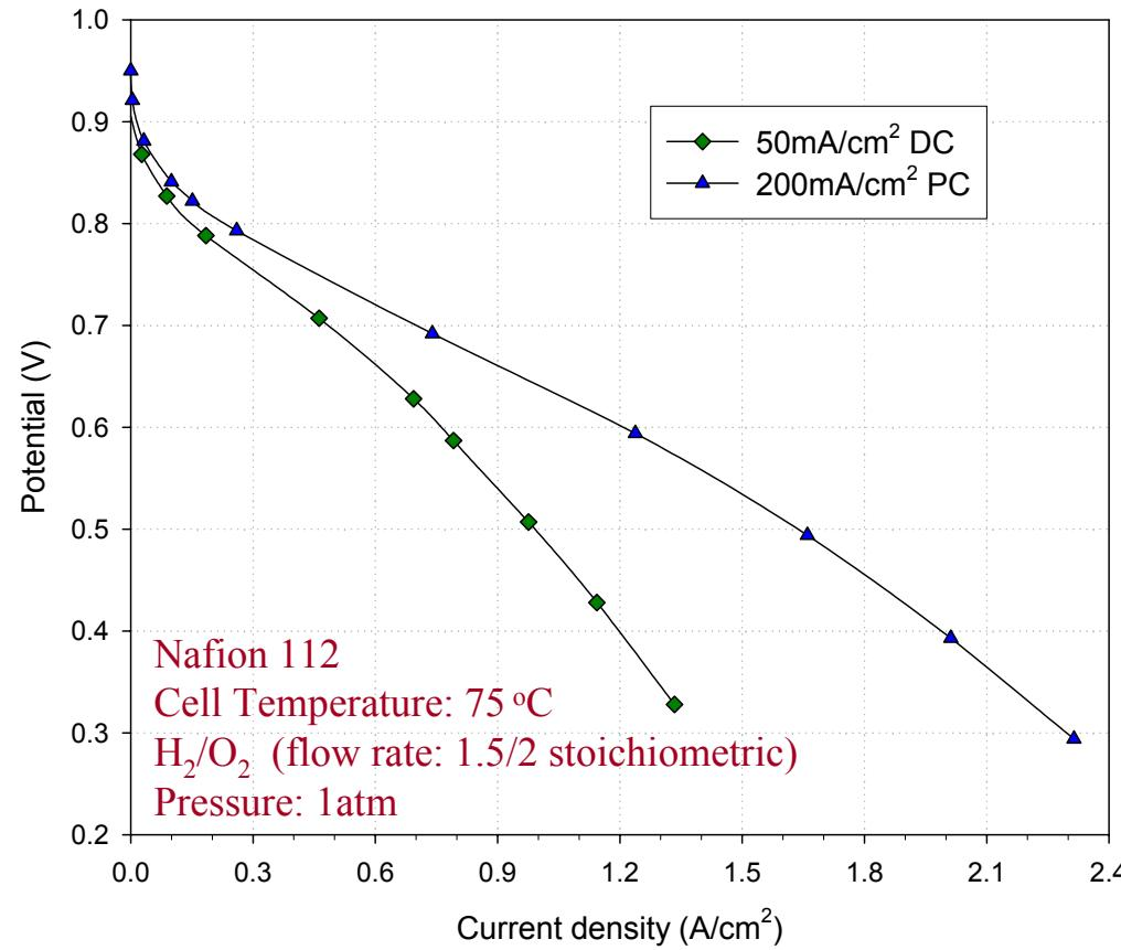
The conditions of pulse electrodeposition:  $200 \text{ mA}/\text{cm}^2$  of peak current density, 5.2ms on time and 70ms off time. Total charge is fixed at  $6 \text{ C}/\text{cm}^2$  on both cases.
