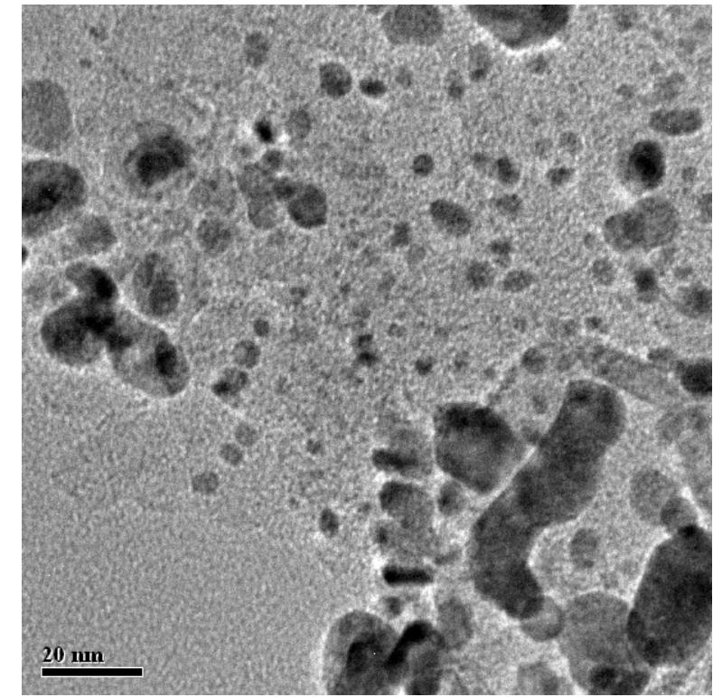
Fig. TEM images of Platinum on carbon nanofibers grown on ACF
