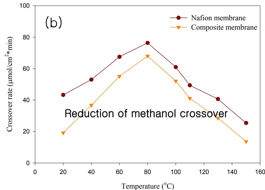
Proton conductivity(a) and methanol crossover rate(b) of the sulfonated polysulfone and sulfonated polysulfone / heteropolyacid –  $\text{SiO}_2$  nanoparticle composite membrane.
