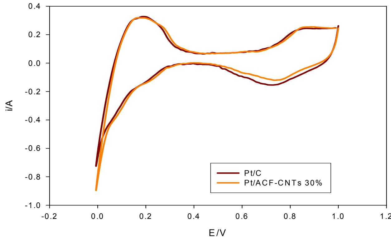
Fig. Cyclic voltammograms of Pt/ACF-CNFs used oxygen
