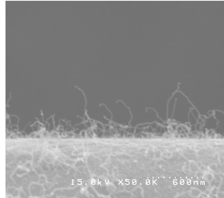
Fig. SEM images of carbon nano fibers grown on ACF
