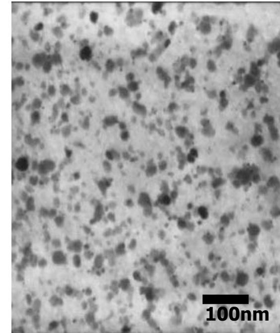
TEM image of heteropolyacid-SiO<sub>2</sub> nanoparticle
