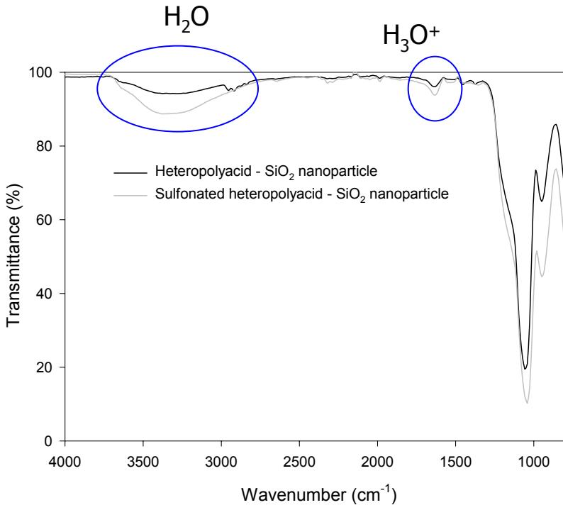
FT-IR spectra of sulfonated heteropolyacid-SiO<sub>2</sub> nanoparticle
