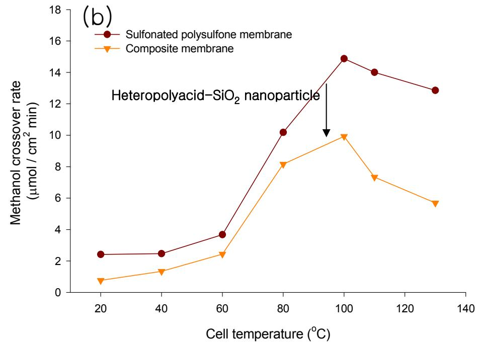
Complex impedance response(a) and methanol crossover rate(b) of the sulfonated polysulfone and sulfonated polysulfone / heteropolyacid – SiO<sub>2</sub> nanoparticle composite membrane.
