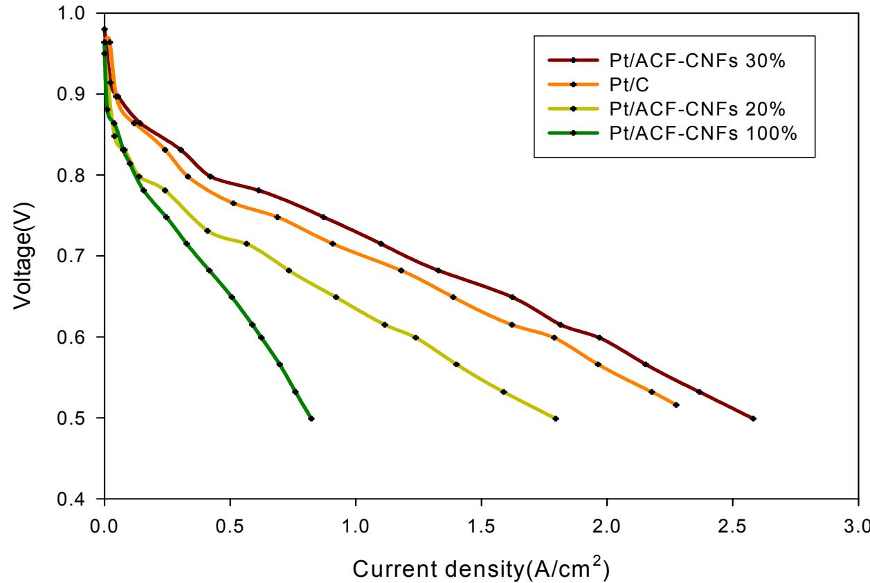
Fig. The performance of Pt/ACF-CNFs used in anode catalyst
