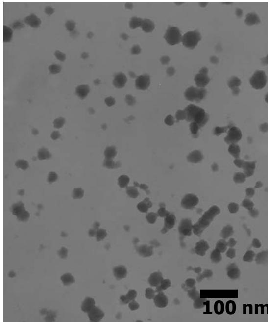
TEM image of heteropolyacid-SiO<sub>2</sub> nanoparticle
