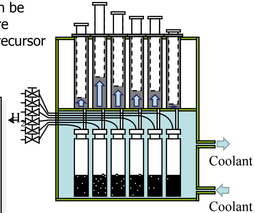
Schematic diagram of simplified HTS test microreactors
