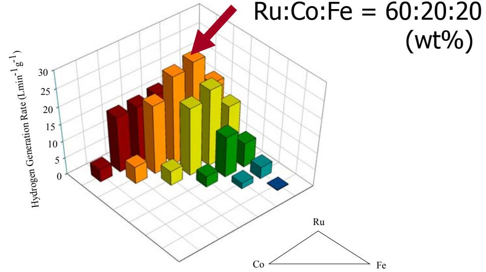
Hydrogen release rate of (a) Ru-Co-Ni, (b) Ru-Co-Fe
