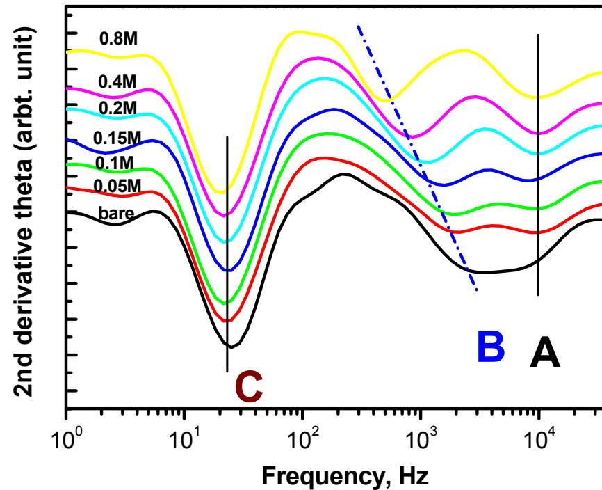
A: pt/electrolyte; B: FTO/electrolyte; C: TiO<sub>2</sub>/dye/electrolyte
