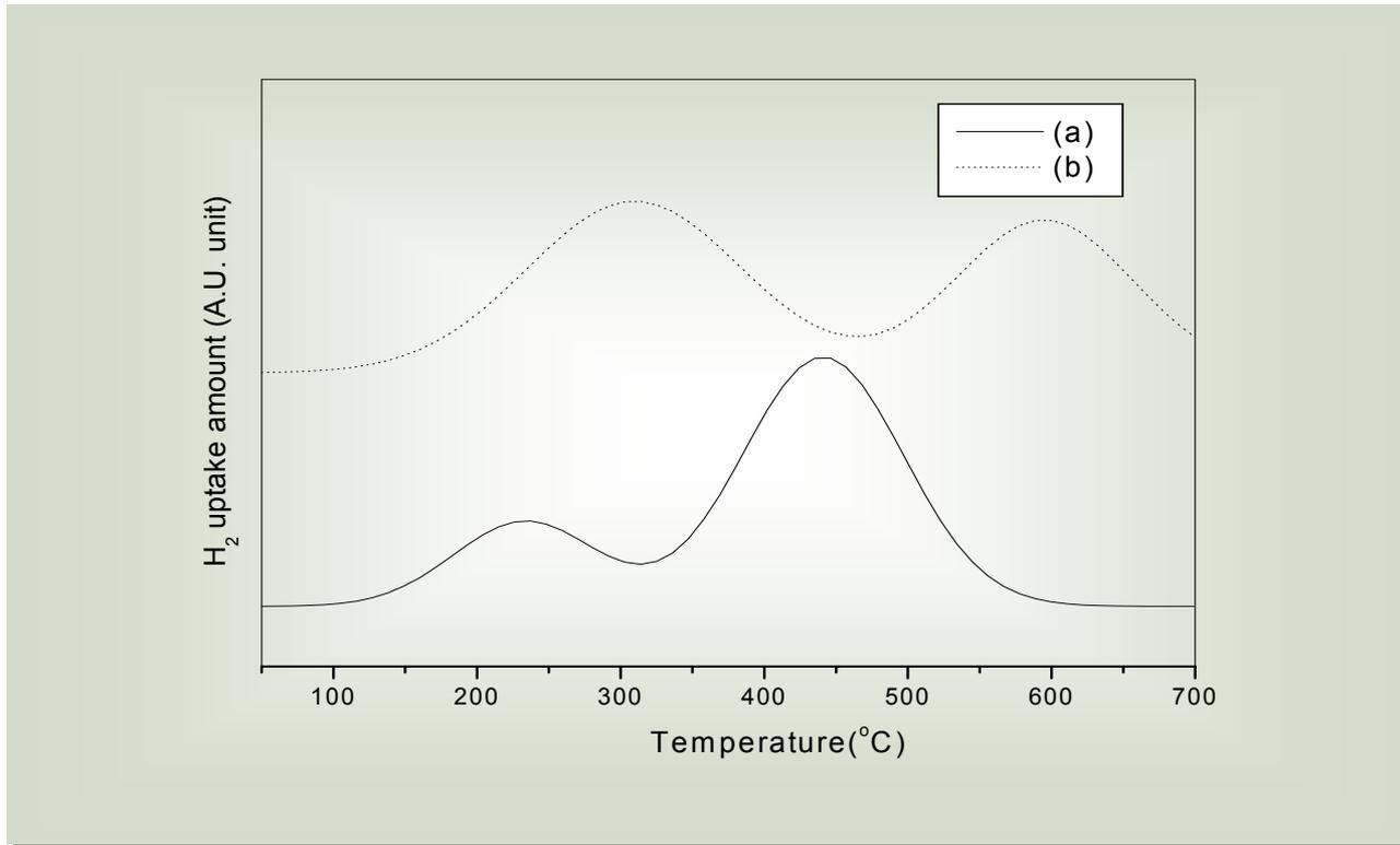
**Temperature programmed reduction of  $\text{La}_{0.8}\text{Sr}_{0.2}\text{Mn}_{1-x}\text{O}_3$  powder after calcination 1000 °C for 4hrs with different starting Materials. (a) nitrate and (b) Oxide**
