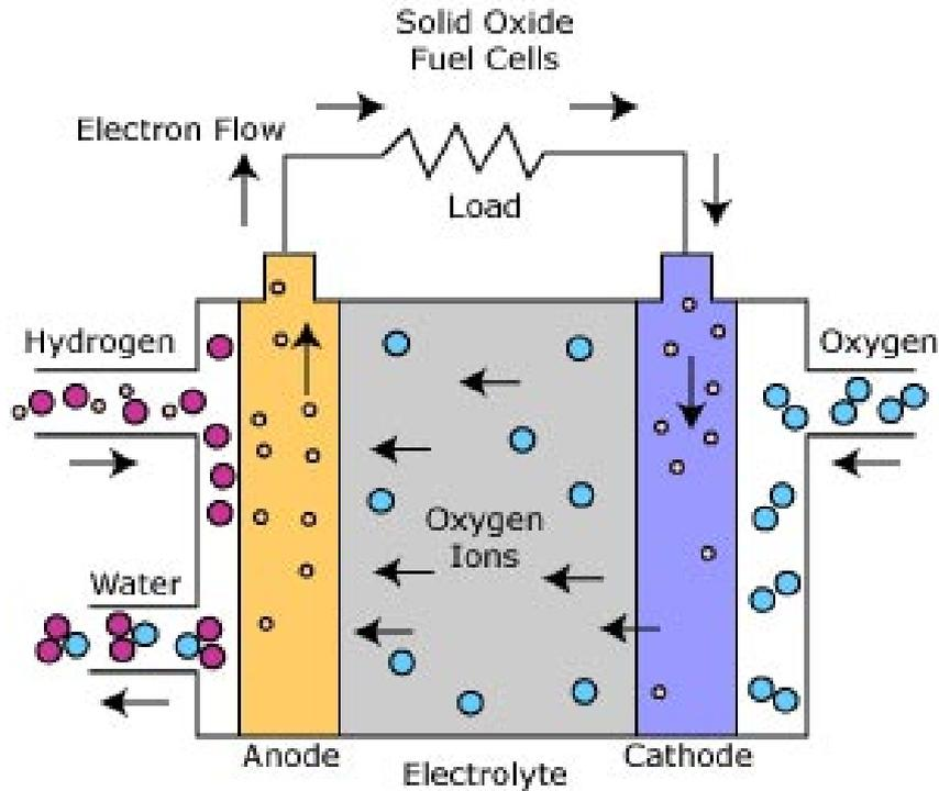
Solid oxide fuel cell is energy conversion device that produces electricity by electrochemical. It operate at high temperature over  $600^{\circ}\text{C}$  with pollution-free technology.
