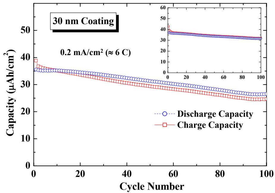
The charge capacity (for Li deintercalation) showed faster deterioration than the discharge capacity (for Li intercalation).
