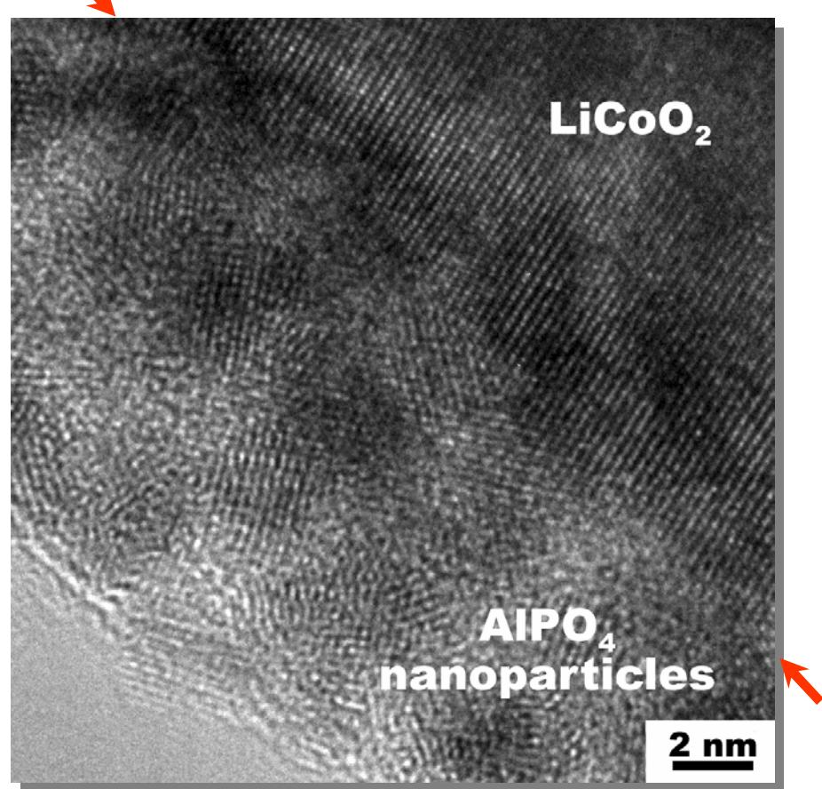
AlPO<sub>4</sub> nanoparticles (~3 nm) embedded in the coating layer (~15 nm).
