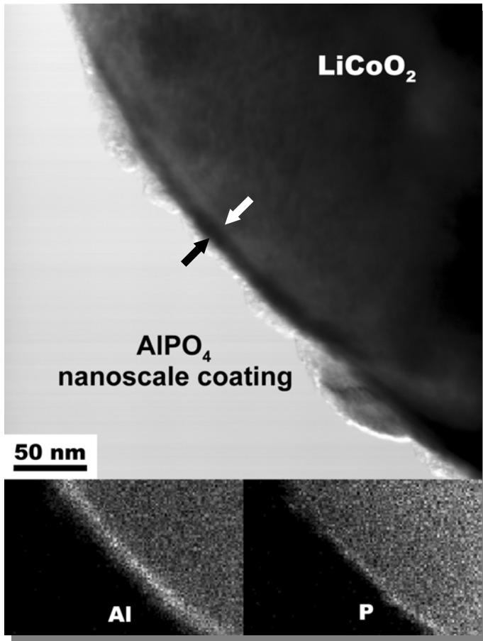
EDS confirms the Al and P components in the nanoscale-coating layer.
