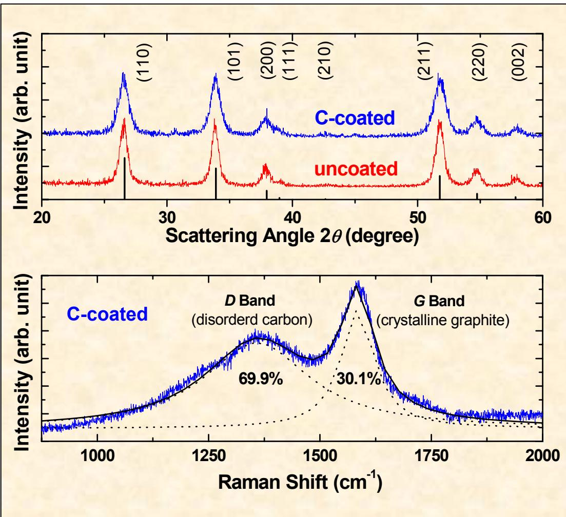
Disordered-carbon-coated SnO<sub>2</sub> nanoparticles
