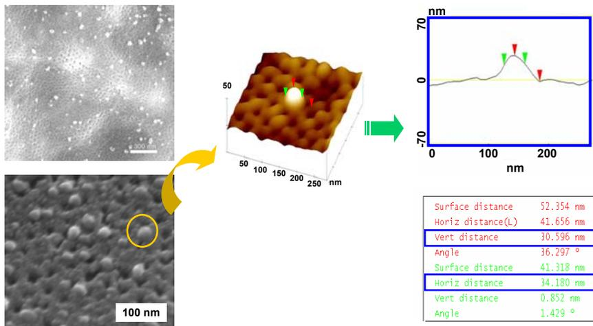
**Shape and size of the particles in the membrane are the same as those of virus (spherical shape & diameter) !!!**
