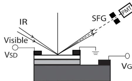
**Fig. 3** In-situ SFG vibrational spectroscopy and electrical characterization of organic field effect transistors during operation.
