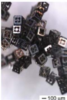
**Fig. 2** 3D self-assembled microcontainers with controlled porosity for cell encapsulation and chemical delivery.
