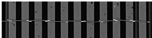
**Fig. 1** Nanowire networks assembled on microfabricated contact pads.
