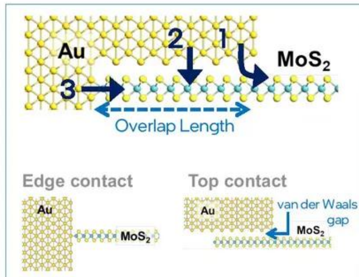
Hybrid contact and its current paths
