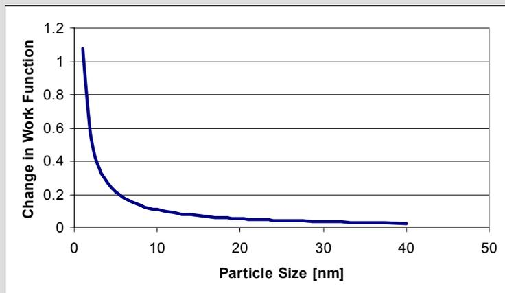
Particle in a Box – Size induced electron levels – Cd Se
