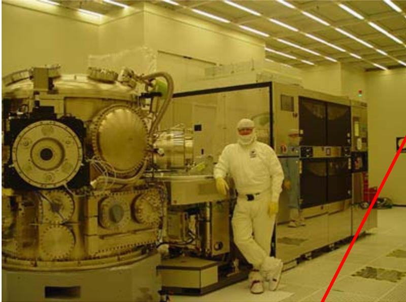
*Intel's Micro-Exposure Tool (MET) for EUV lithography development*
