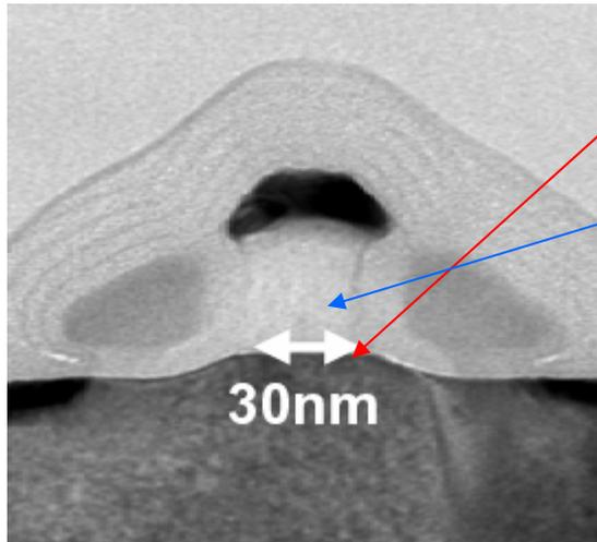
Growth of 1 nm thick oxide must be uniform across 300 mm wafer
