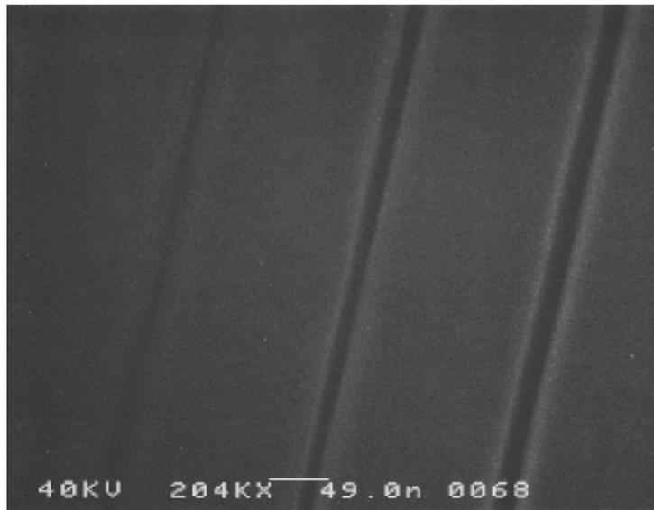
*Small lines ( $\geq 6$  nm) obtained in PMMA*
