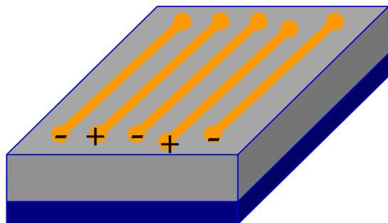
2. Nanotubes align on negatively charged nanowires via noncovalent, electrostatic attraction
