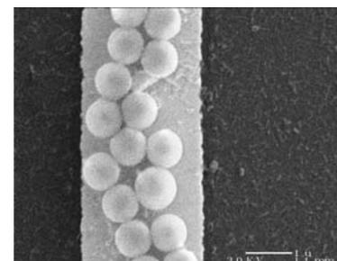
Guided self assembly of particles onto Au wires (Busnaina, NEU, 2003)
