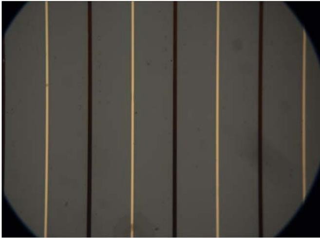
CNT on 2 micron Au wires, black wires are positive charged and yellow negative
