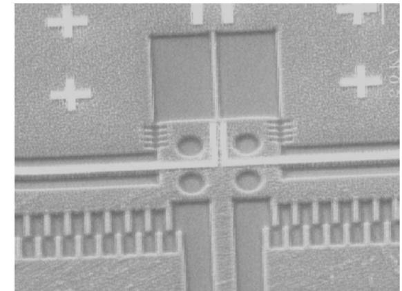
**Innovative MEMS devices characterize nanowires (also nanotubes, nanorods and nanofibers) and conduct accelerated lifetime testing allowing rapid mechanical, electrical, and thermal cycling during UHV SPM observation**
