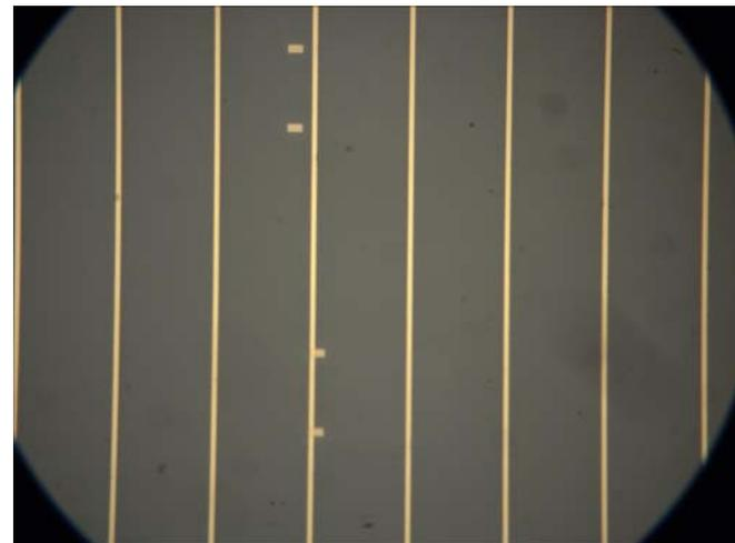
50nm nanowires (nanotemplates) connected to 2 micron wires (nanowires cannot be seen in optical microscope)
