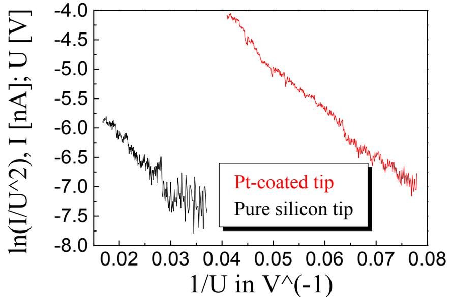
Turn-on field emission for the Pt-coated tip has demonstrated with an extraction voltage as low as 15 V
