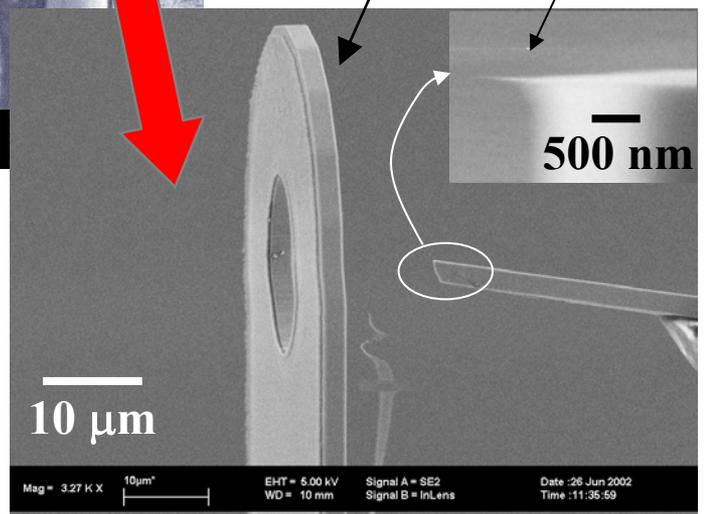
A tip-extraction electrode distance of 10 µm achieved by LEGO microstage
