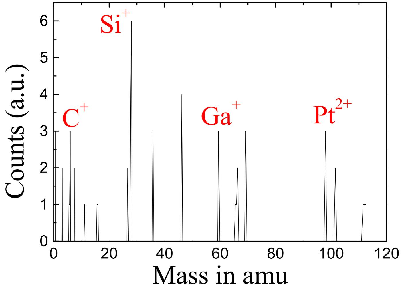
$Si^+$  and  $Pt^{2+}$  peaks of Pt-coated tip at mass to charge ratio of 28 and 97.5
