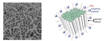
Left: Porous silicon nanoparticles by TEM. Nominal particle size is 200nm. Right: Porous silicon nanoparticle design.
