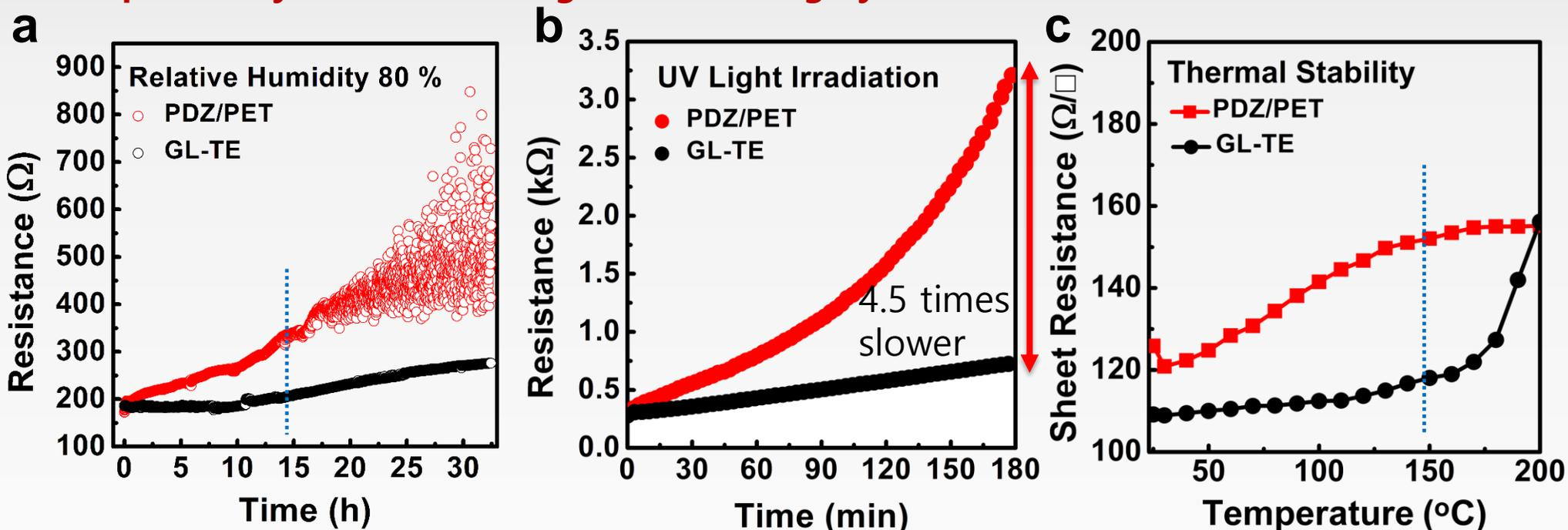
a, b) UV stability and Relative humidity test according to the resistance change while the samples were exposed to the radiation of an Xe lamp at 254 nm wavelength and humidity 80% respectively.
