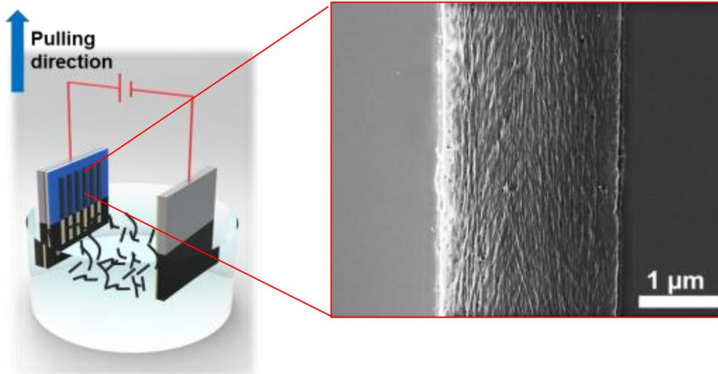
✓ Alignment of Single Walled Carbon Nanotubes can be controlled during printing process
