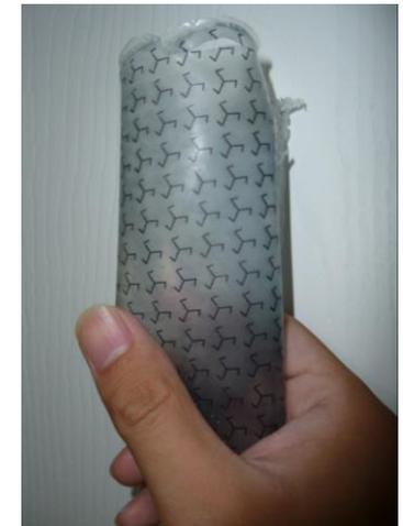
Printing of mm Scale Chiral Metamaterial
