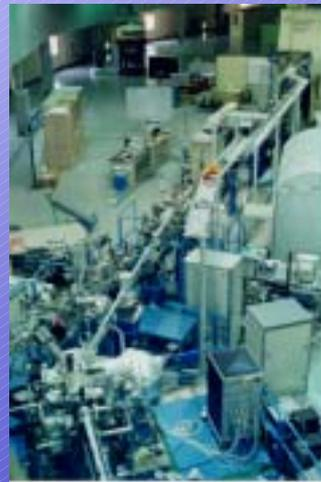
Synchrotron-radiation photoelectron spectroscopy system
