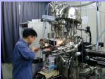
4 K Scanning Tunneling Microscope
