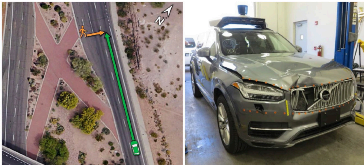
Figure 1: 2018 fatal crash of a highly automated vehicle deployed by Uber in Arizona. Left: Path of pedestrian (orange) and vehicle (green). Right: post-crash view of vehicle. Source (NTSB 2019).
