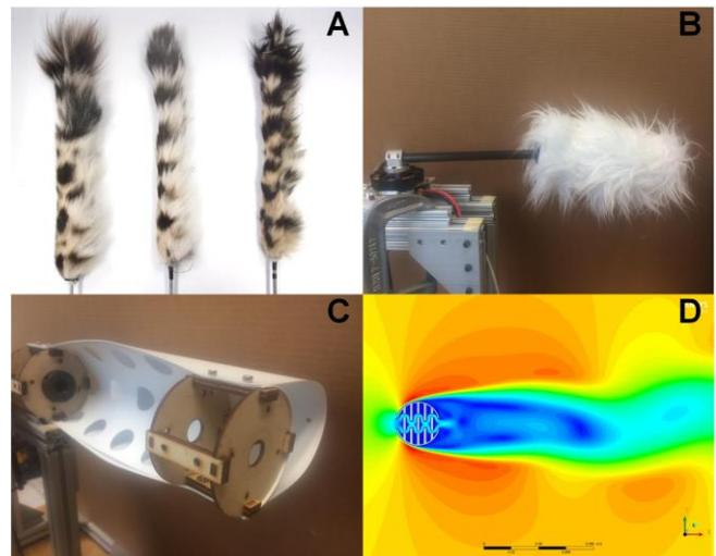
Fig. 1. (A) Three cheetah tails were dynamically tested in a wind tunnel. (B) The biomimetic tail developed attached to the mechanical rig. (C) The plastic tail with slots for creating drag. (D) CFD simulation snapshots of the first 1 minute of a slotted design for the tail.
