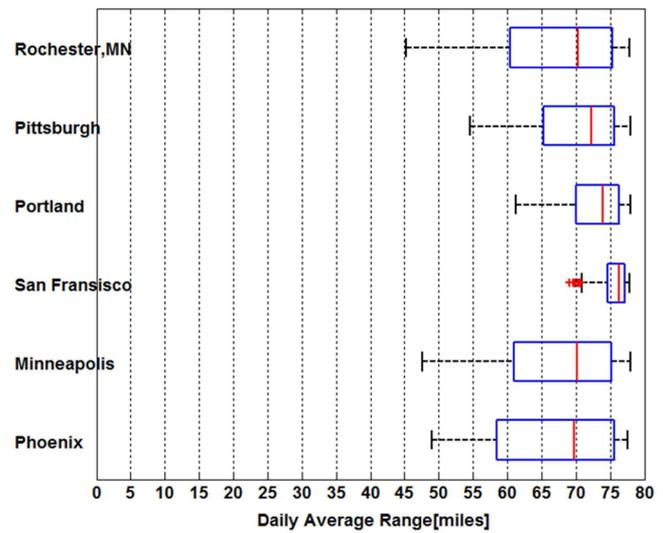
Figure 2. Box plot of daily driving range distributions for selected cities. Red lines indicate median range; blue boxes capture the 2nd and 3rd quartiles across days of the year; the whiskers extend to the most extreme data points that are not considered outliers, and the red + symbols indicate outlier days.
