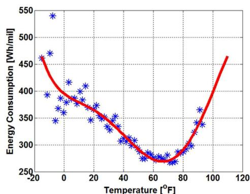
**Figure 1.** Nissan Leaf energy consumption per mile versus ambient temperature. The blue stars correspond to data points obtained by converting FleetCarma range data to energy consumption. The red curve is the polynomial fit given by eq 1.
