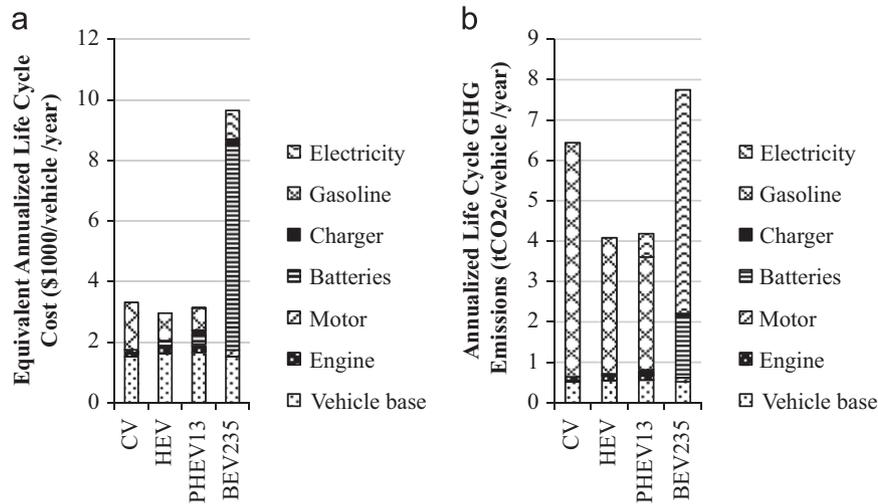
Fig. 4. Breakdown of (a) equivalent annualized life cycle cost and (b) life cycle GHG emissions for four independently cost-optimized vehicle designs.
