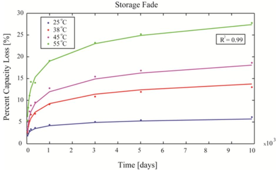
**Figure 4** – Capacity Fade at Storage-Data and Fit (Used with permission [24])
