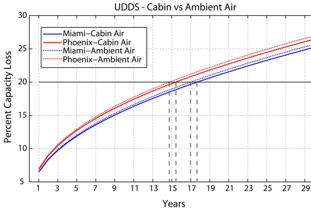
Figure 8. Cooling medium comparison for driving with UDDS- Cabin air vs ambient air
