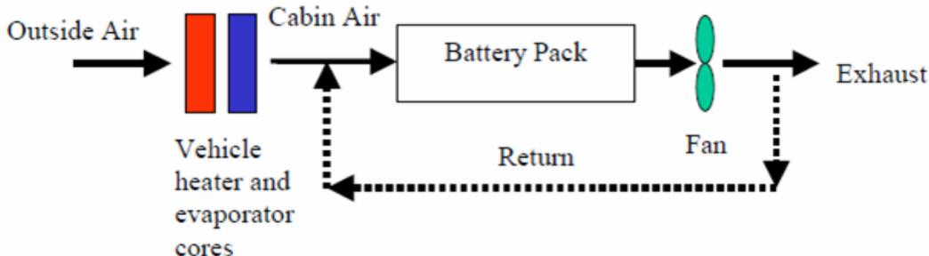
Figure 1. Air cooling thermal management system [21]
