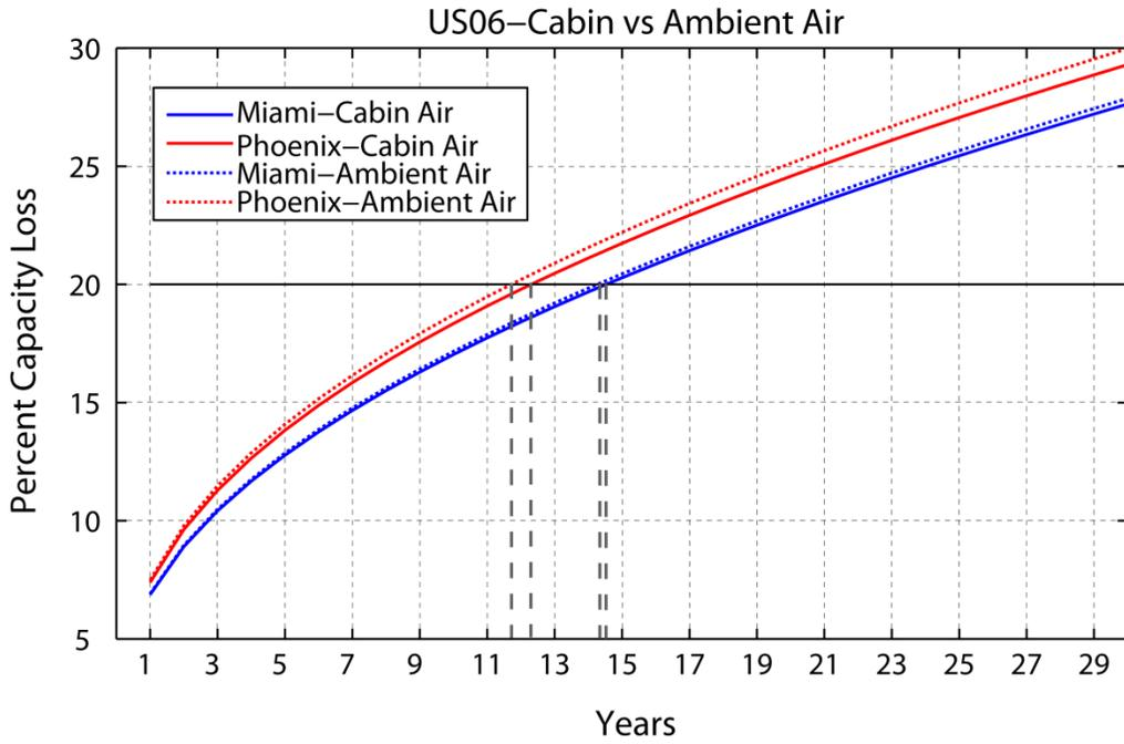
**Figure 9.** Cooling medium comparison for driving with US06- Cabin air vs ambient air
