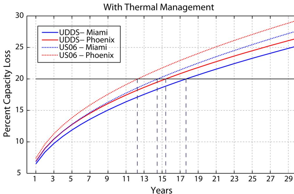
**Figure 6.** Capacity fade comparison for driving with UDDS and US06- with thermal management
