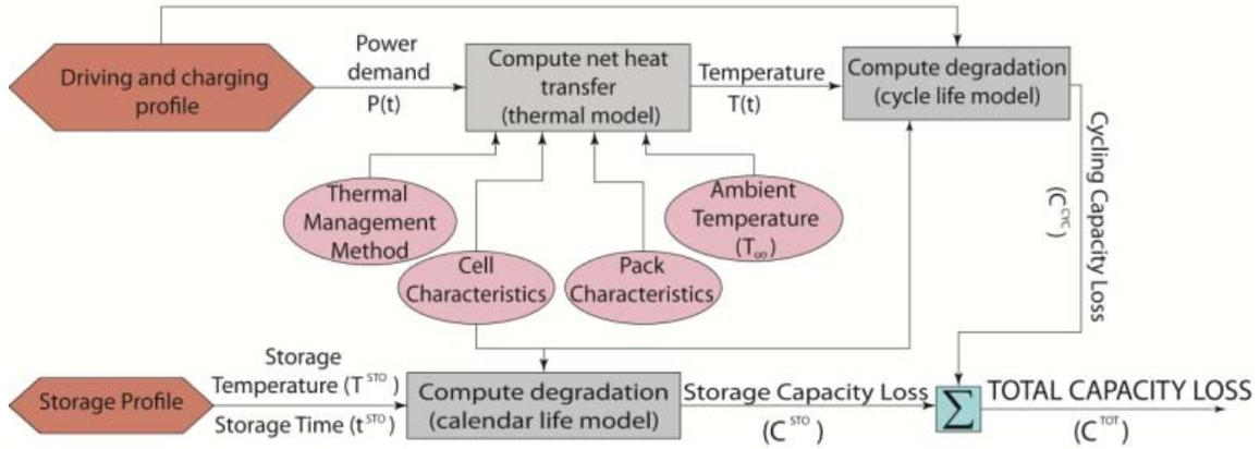
**Figure 5** - Schematic view of simulations to calculate battery life (Used with permission [1])
