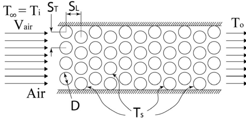
**Figure 2.** Staggered cell arrangement inside a module (Used with permission [1])
