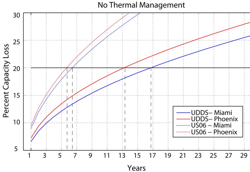
Figure 7. Capacity fade comparison for driving with UDDS and US06- no thermal management
