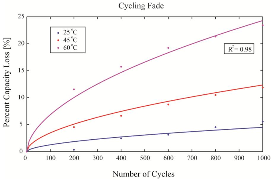
**Figure 3** – Capacity fade with cycling-Data and fit (Used with permission [24])
