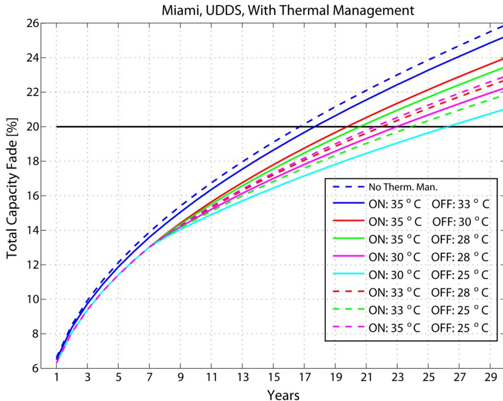
**Figure 10.** Capacity fade in Miami with UDDS- Comparison of fan on-off temperatures
