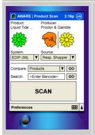
**Project**: Develop a functional PDA barcode scanner prototype that will provide (1) producer-level data about the scanned product from Co-op America's Responsible Shopper database and (2) product-level data for the products compiled by Katie Kerfoot (ME490 project).
