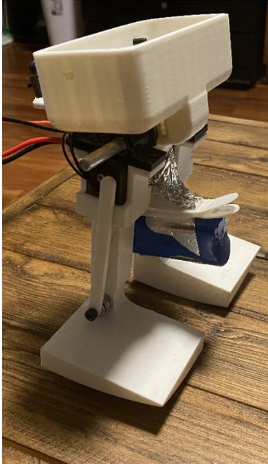
The walker to the left utilizes the principles of passive dynamics and 2 servos that push the legs in and out. The servos are used to excite the wobble, to push off, and gain leg clearance. The feet are curved in the same way as shown previously. Also, the hip is shift forward to make the robot lean forward.
