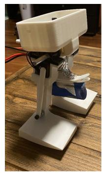
The walker to the left utilizes the principles of passive dynamics and 2 servos that push the legs in and out. The servos are used to excite the wobble, to push off, and gain leg clearance. The feet are curved in the same way as shown previously. Also, the hip is shift forward to make the robot lean forward.
