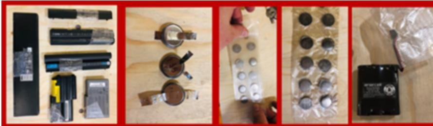
Batteries taped for recycling
