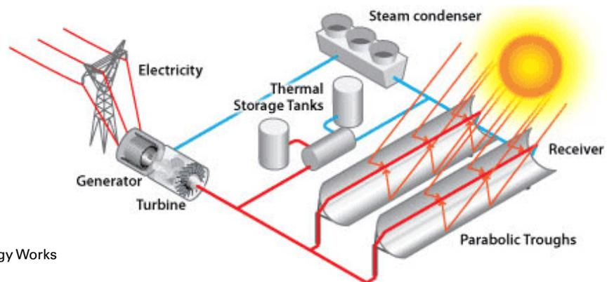
Figure 5a: How Solar Thermal Energy Works
