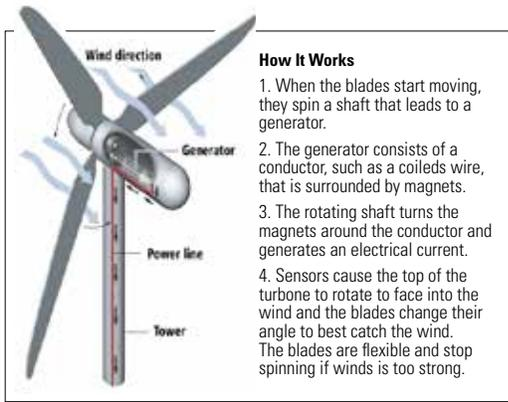
**Turning Wind into Electricity:** Wind power is the fastest-growing energy source in the world. Turbines powered by wind are mounted on towers 100 or more feet above the ground, where the wind is faster and less turbulent.
