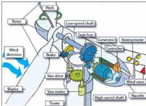
Figure 4: How Does a Wind Turbine Work?
