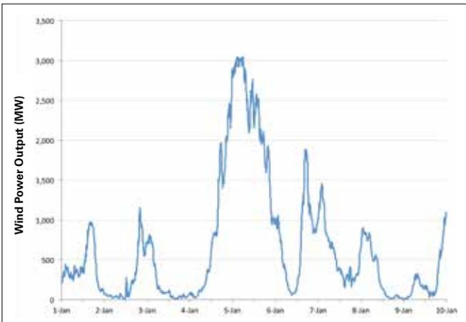
Figure 7: 5-Minute Wind Power Output in BPA, 1/1/2012 to 1/8/2012.
