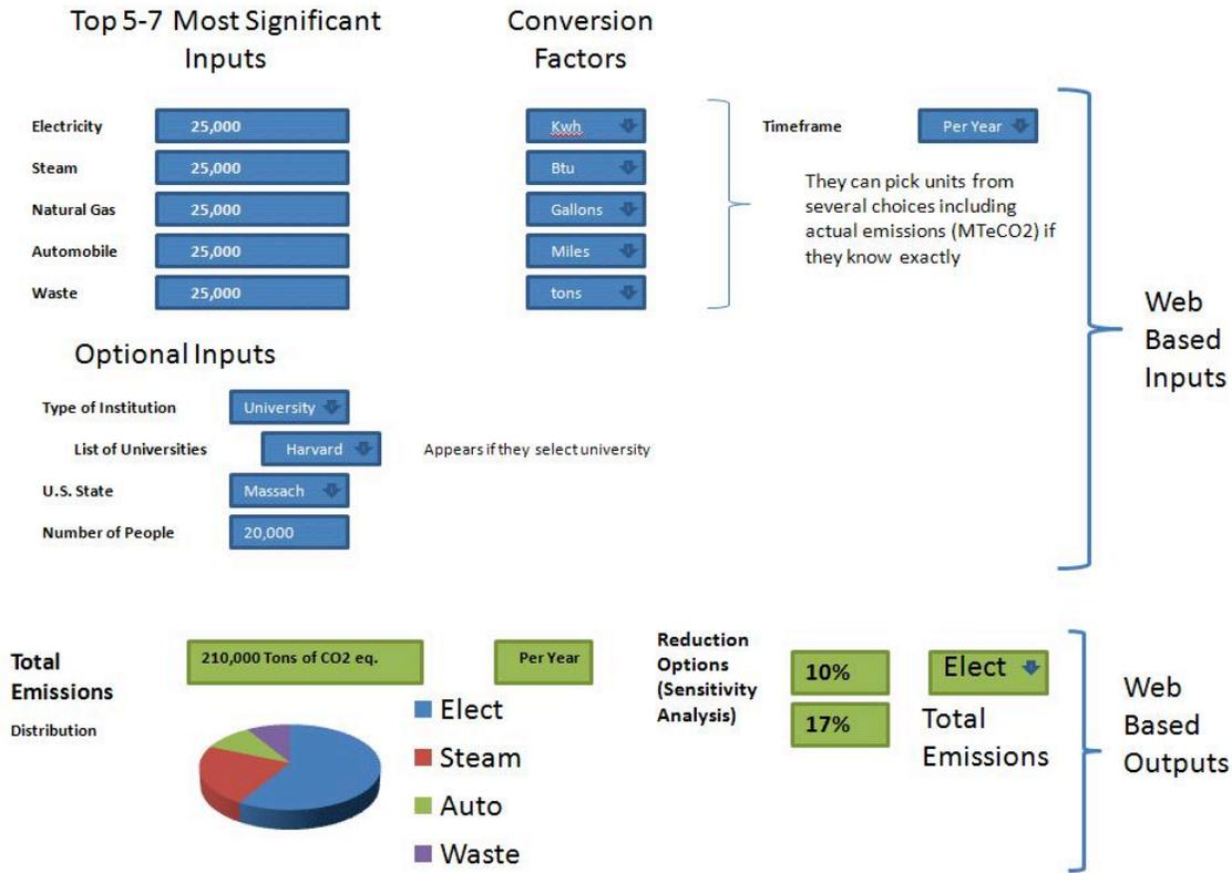
Figure 2.A.1 – Conceptual Design of Web/Excel Emissions Estimator Application
