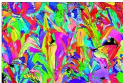
ON THE COVER: Electron backscatter diffraction inverse pole figure map of a cross sectioned 316L stainless steel cube, which was additively manufactured with laser powder bed fusion (where the build direction is vertical)
