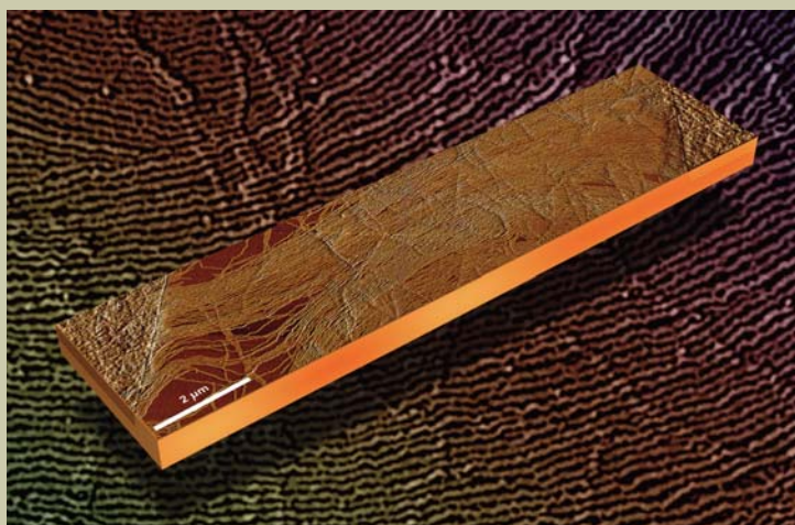
Figure 2: Individual regioregular polythiophene nanofibrils spanning a 10 \mu\text{m} channel of an organic field-effect transistor with planarized contacts.
