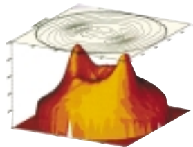
◀ X-ray pole figure from a rolled titanium aluminide alloy
